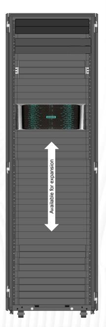
Production Network Module (2) HPE Aruba 8325-32Q (Leaf/Border) Management Network Module (2) HPE Aruba 6300M Control Plane (3) HPE ProLiant DL325 Gen10+
